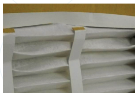
If the filter looks like this after you take it out of its packaging, don't install it.
