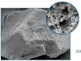
SEM of Activated Carbon Particle
