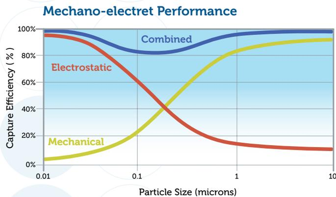
*The best filter is a good mechanical filter augmented with an electrostatic charge*
