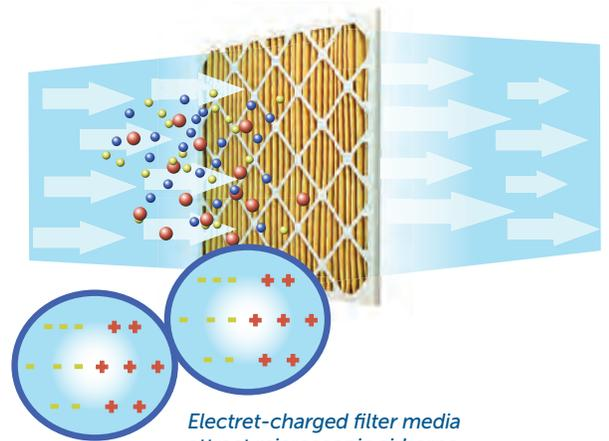
*Electret-charged filter media attract microscopic airborne particles in much the same way a magnet attracts iron particles.*
